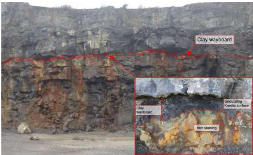
Figure 3.15: Clay wayboard on the quarry face at Lackagh Quarry
