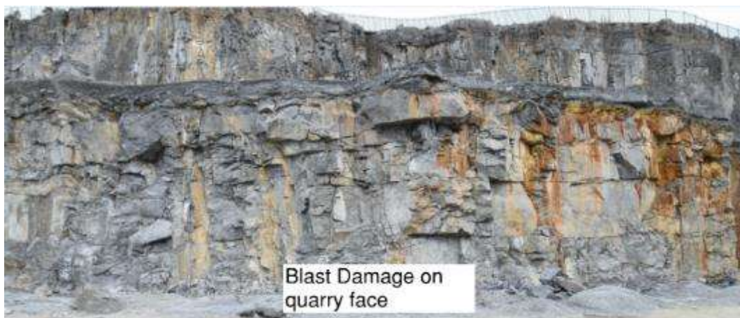
Figure 3.17: Blast damage on quarry face
