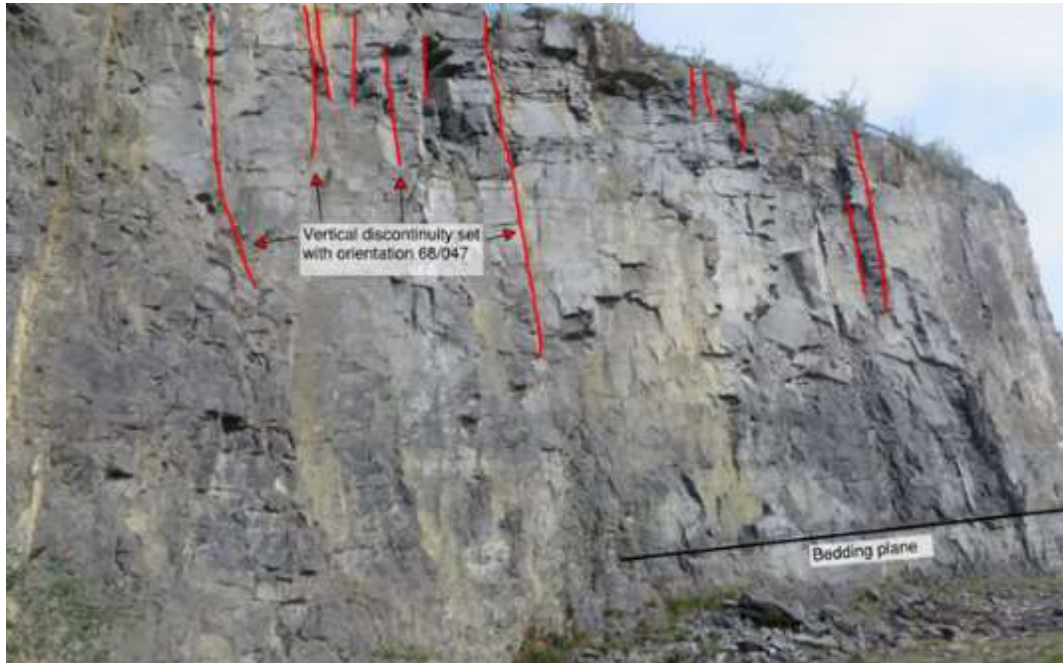
Figure 3.16: Exposed discontinuities on the upper bench
