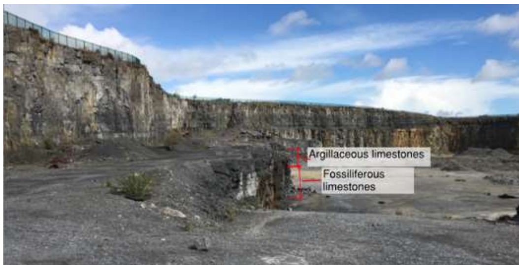
Figure 3.14: Cyclical sequence of Limestones at Lackagh Quarry
